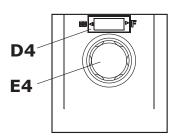
Once you have chosen the cleaning cycle to clean the cooking chamber, all you need to do is to confirm it by pressing the program knob **E4**.
